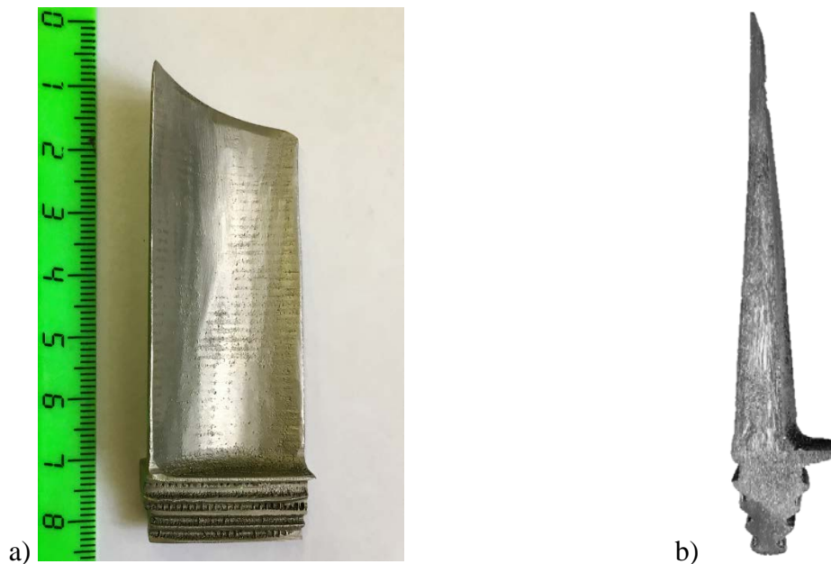
Fig. 9. The photograph of the produced blade (a) and its microstructure (b).
