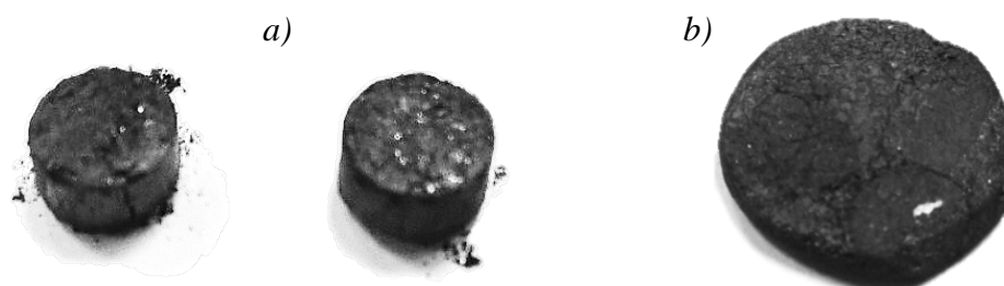
Fig. 3. Solid samples obtained: a) by cold pressing, b) by hot vacuum pressing
