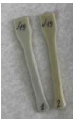
Fig. 3. Specimens 1 and 2 with the oil contents of 20 and 25 weight parts, respectively, for SIS VECTOR 4111NS
