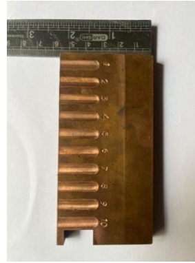
Fig. 12. A section removed for analysis from as-built CuCrZr
