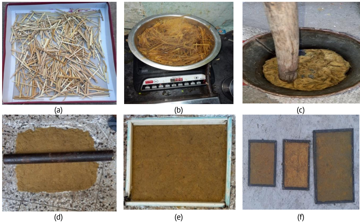
Fig. 1. Development of sheets from rice straw fiber
