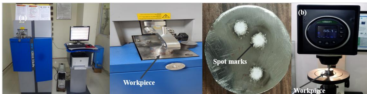
Fig. 1. Spectrometric analyses (a), hardness tester (b)
