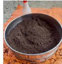
Fig. 5. Combine the cocopeat and cement mixture
