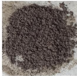
Fig. 4. Cocopeat after mixing with 100 g of cement
