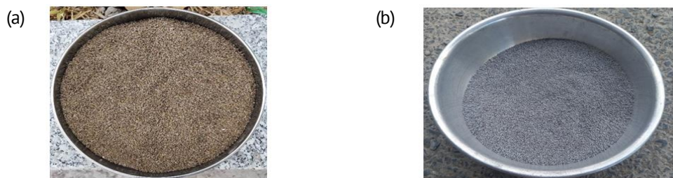
Fig. 6. Cocopeat hardened with cement: (a) finished product remaining on 0.63 mm sieve, (b) finished cocopeat granules have been hardened with cement
