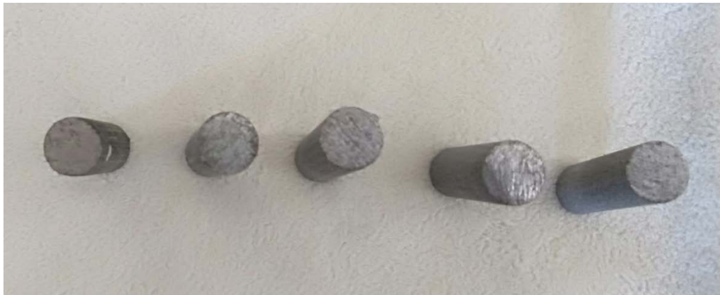
Fig. 3. The macro images of the pins (Mg, Mg+2%Ti, Mg+4%Ti, Mg+6%Ti, and Mg+8%Ti from left to right) after wear tests
