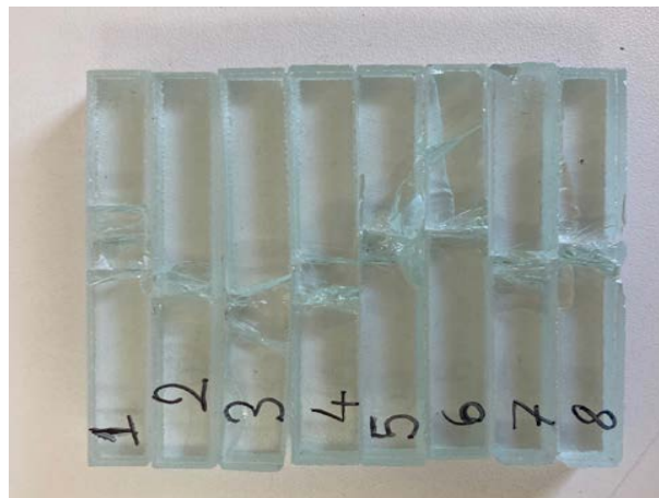
Fig. 3. Laminated glass specimens after impact
