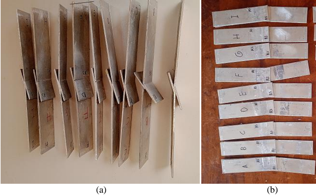
Fig.10. Different modes of fracture: a) single lap; b) double lap
