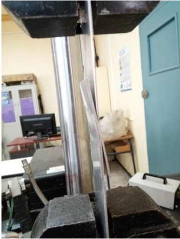
Fig.9. Shear specimen during the tensile test
