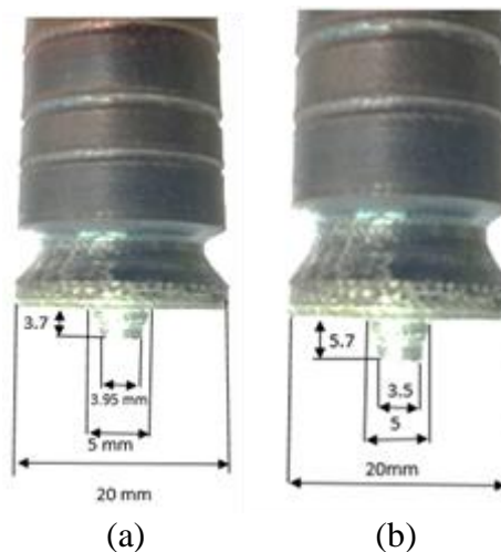
Fig. 2. Types of tools used for FSLW: a) single lap, b) double lap
